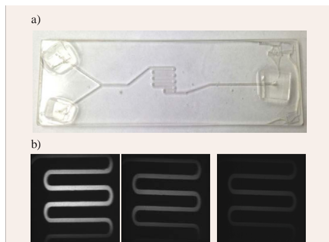
Figure 1 Microfluidic device for the Paal-Knorr pyrrole synthesis. a) A device fabricated with quartz slides and NOA 81 UV optical adhesive. b) Micrographs of caffeine standards in the microchannel for calibrating the UV imaging system for online reaction monitoring. From left to right, the concentrations are 0, 500, and 1000 ppm, respectively. The microchannel became darker and darker due to the increased absorbance at higher caffeine concentrations. The background was completely dark because the stray light was absorbed by the microchannel wall formed by the UV-curable adhesive, which served as a built-in optical slit. The width and depth of the microchannel are 300 and 250 \mu\text{m} , respectively [39].
